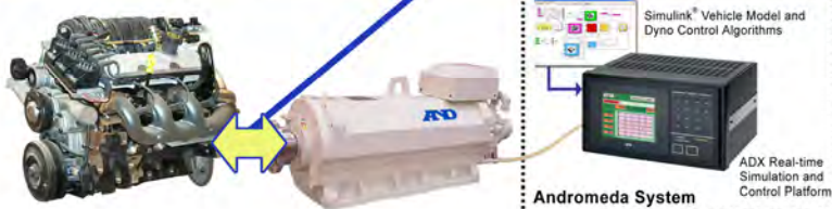
The Andromeda system in an engine-in-the-loop configuration
