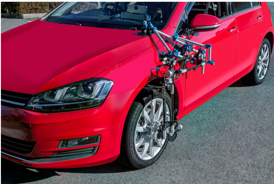
The WPS Wheel Position Sensor measures the six-component position of a wheel in dynamic conditions.
